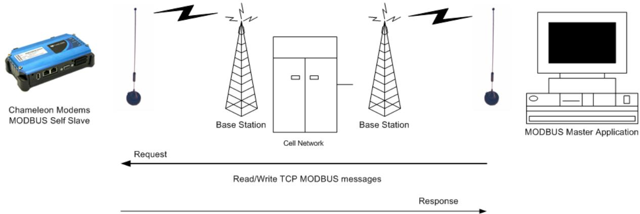
A MODBUS Master Application can “read” and “write” to a CTM modem configured as a MODBUS Self Slave. See [http://www.cypress.bc.ca/modbus\\_messages\\_ctm200.html](http://www.cypress.bc.ca/modbus_messages_ctm200.html) for example read/write messages to send from the MODBUS Master Application to the CTM modem.
