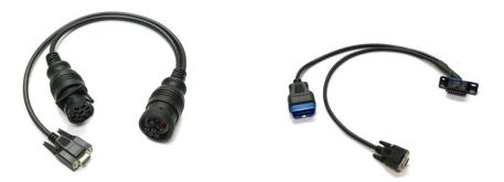
The Y-Cable is meant to take the place of the factory connection located in the steering column area of the vehicle. Remove the bulkhead connector from the vehicle and connect it to the mating end of the Y-cable. Replace the bulkhead connector with the other end of the Y-cable in the same place as the original connector and tuck wiring harness in behind dash.
