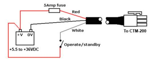
The power cable has three wires:
